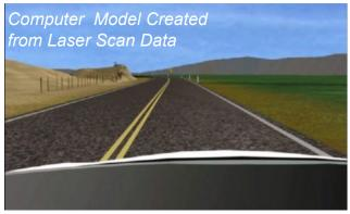
PSI then used construction plans and photos of the original highway, combined with additional analytical software, to modify the working model to accurately recreate the roadway as it existed during the collision and before it had been remodeled. PSI then programmed the vehicle motion up to and after impact using the expert's calculations developed from the physical evidence at the site.
