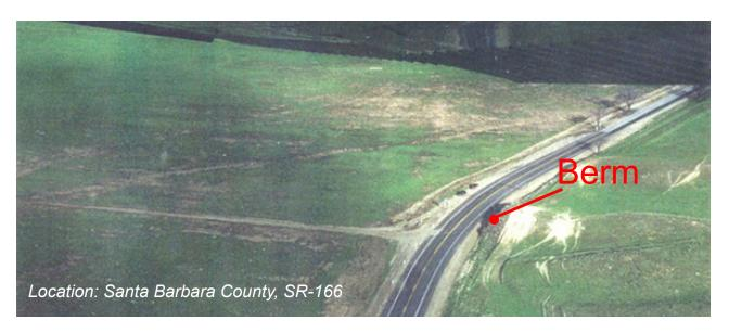
The berm was large and irregular making it difficult to mathematically determine when the drivers were able to see each other. The police would not allow the highway to be closed and the highway had been modified since the accident.
